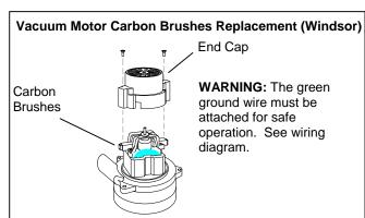
If armature commutator is grooved, extremely pitted or not concentric, the motor will need to be replaced or sent to a qualified service center.
